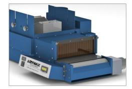
Two LED Floods Mounted in a UVCS Conveyor
