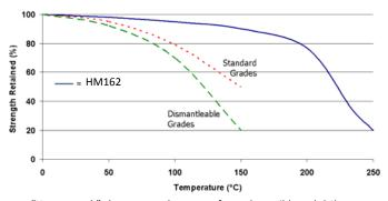
"Hot strength" shear strength tests performed on mild steel. 24hr cure at room temperature and conditioned to pull temperature for 30 minutes before testing.
