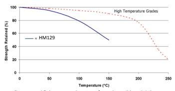
"Hot strength" shear strength tests performed on mild steel. 24hr cure at room temperature and conditioned to pull temperature for 30 minutes
