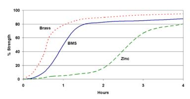
Cure times are typical at 23°C. Copper and its alloys will follow the faster cure while oxidised or passivated surfaces like stainless steel will tend towards the slower curve. Lower temperatures or large gaps will tend to extend the cure time. To reduce the cure time the use of Permabond A905, ASC10, or heat can be considered.
